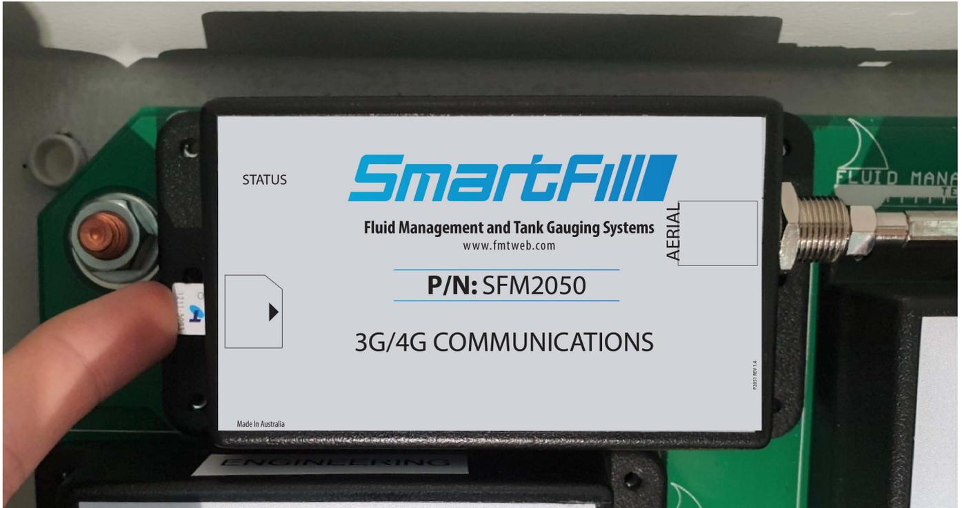
Figure 2.21: Installing SIM
