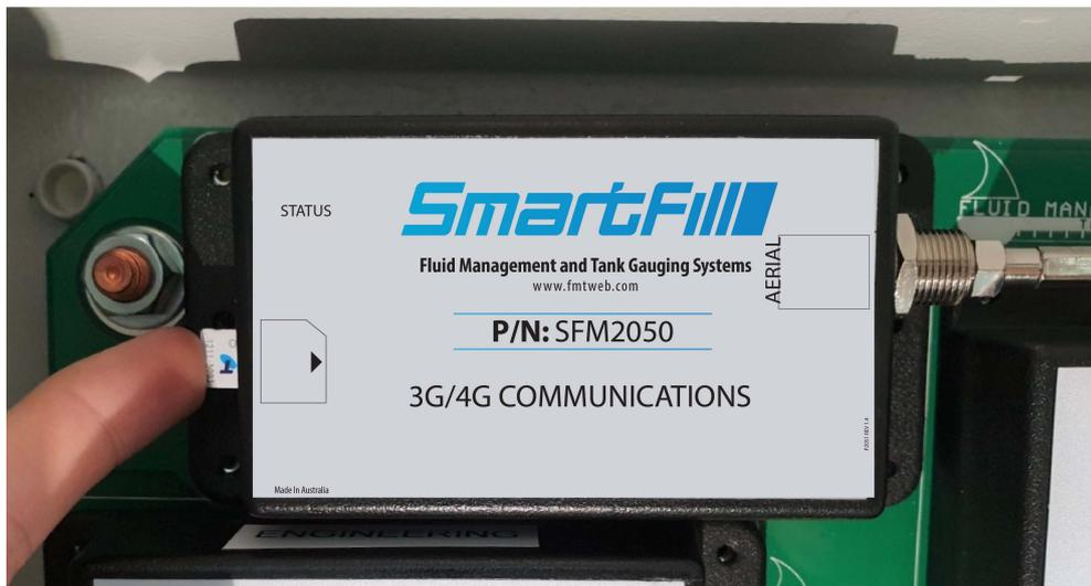
Figure 1: Installing SIM
