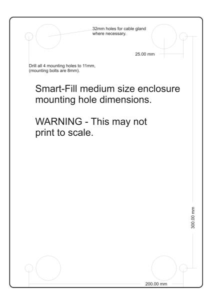
Figure 1: SmartFill Model A1001 Enclosure Dimensions
